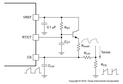
Figure 27. Slope Compensation Circuit
