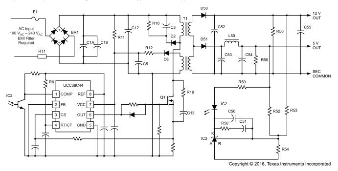
Figure 29. Typical Off-Line Application
